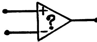
There are two inputs and one output. The inputs can be continuous voltages from, say, a scale of 0-10. The output however is allowed only two conditions: ON or OFF. The appropriate condition is determined by comparing the values of the two inputs. If the + input value is greater than the - input value the output is ON; If the + input is the same as or less than the - input the output is OFF. A typical circuit used for this function is the u710 integrated circuit, about the size of a dime.
