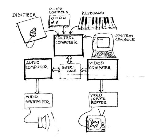
mon interface. The audio and video sections run their own programs, operating the audio synthesiser and the video frame buffer, respectively. The actual hardware implementation will rely heavily on 8 bit micrprocessors, running in parallel. This gives the system more power than a single 16 bit machine could give.
