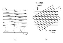
Fig. 2. Video raster with arrows indicating the direction of scanning. Solid lines correspond to when the electron beam is on; the dashed lines when the beam is off during the *retrace* time. (b) Since the raster defines the horizontal, in a feedback system the relative orientation as shown of the camera and monitor is an important control parameter.
