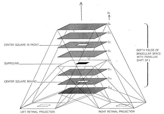
AUTOMAP-1 is a computer program that compiles a threedimensional contour map from two-dimensional stereoscopic images. The program compares left and right fields point by point and subtracts the brightness of each point from its counterpart.
