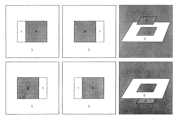
STEREOSCOPIC PRINCIPLE is simply that identical areas that appear in both fields must be shifted horizontally with respect to each other. Because these areas are themselves randomdot patterns they cannot be seen monocularly against a randomdot surround. In these diagrams A identifies the area common
