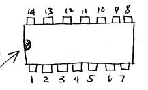
Knotch or dot indicates installation direction.
