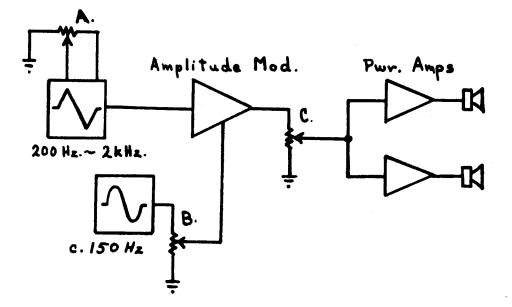
A. B. and C. are linear center-tapped servopotentiometers with weighted shafts.
